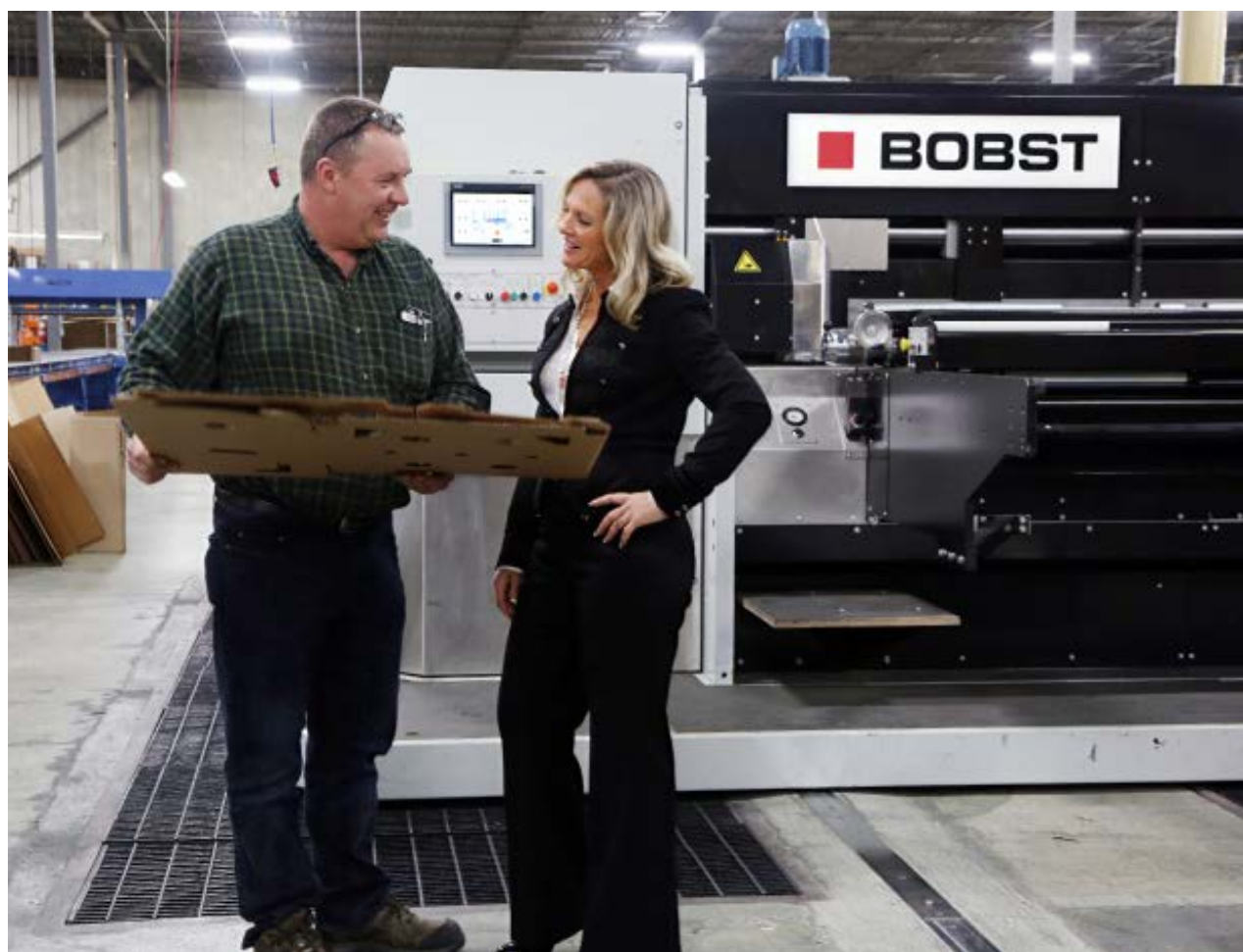
Royal Containers plant manager Henry Lambert (left) and company president Kim Nelson examine a sample of intricately die-cut corrugated sheets coming off the BOBST flexo folder gluer machine behind them.
