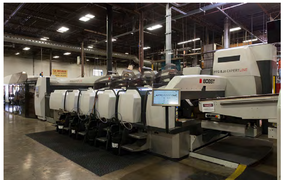
Manufactured by Bobst, the recently-installed 8.20 EXPERTLINE flexo folder-gluer has enabled the Mitchel-Lincoln boxmaking facility to achieve record output speeds.
