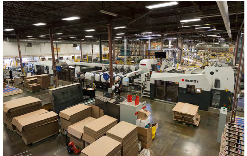
Strategically positioned right at the center of the action of Mitchel-Lincoln's busy 220,00-square-foot production facility, the 8.20 EXPERTLINE flexo folder-gluer manufactured by Bobst has enabled the plant to achieve dramatic productivity improvements.
