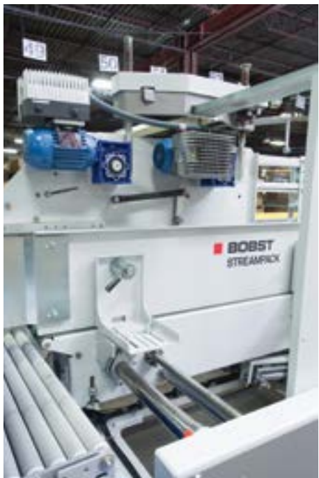
The STREAMPACK batch collector installed at the end of EXPERTFOLD line.
