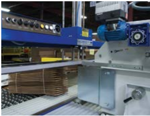
An inline MOSCA strapping machine (left) makes the compressed bundles of corrugated boxes coming off the STREAMPACK batch collector ready for shipment.
