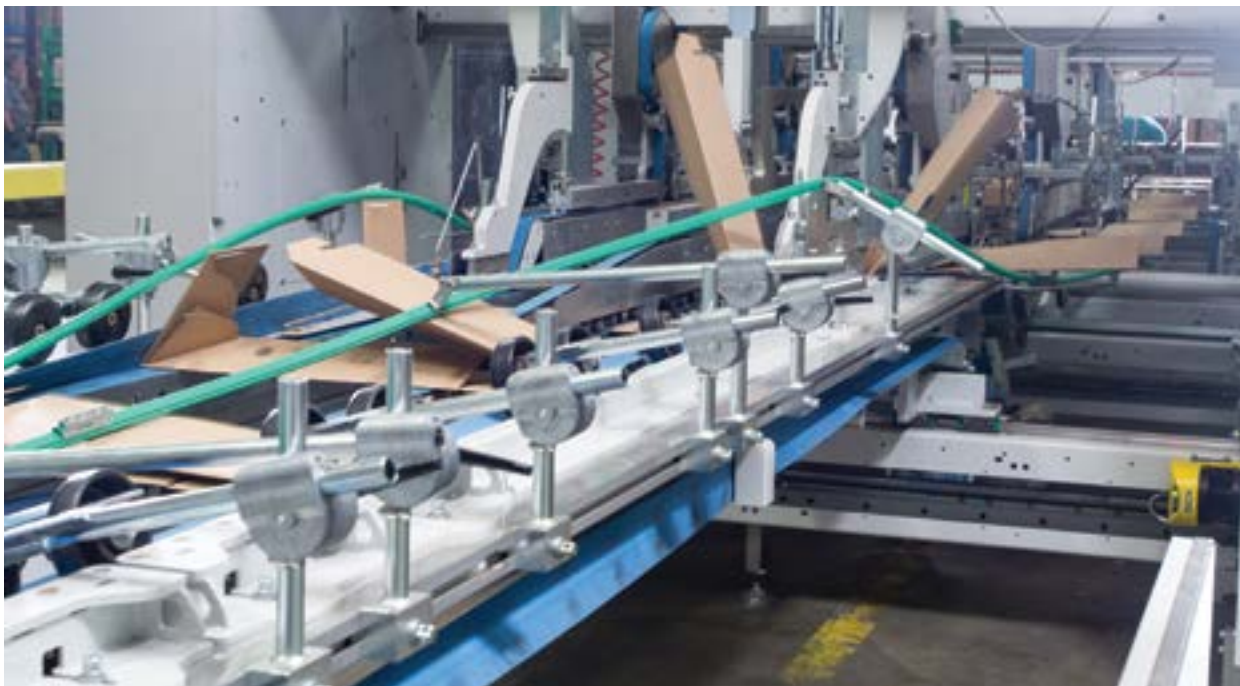
The newly-installed EXPERTFOLD folder-gluer from BOBST has enabled the Gerrity plant to run a broader range of complicated and narrow box designs at very robust throughput speeds of up to 6,000 boxes per hour.
